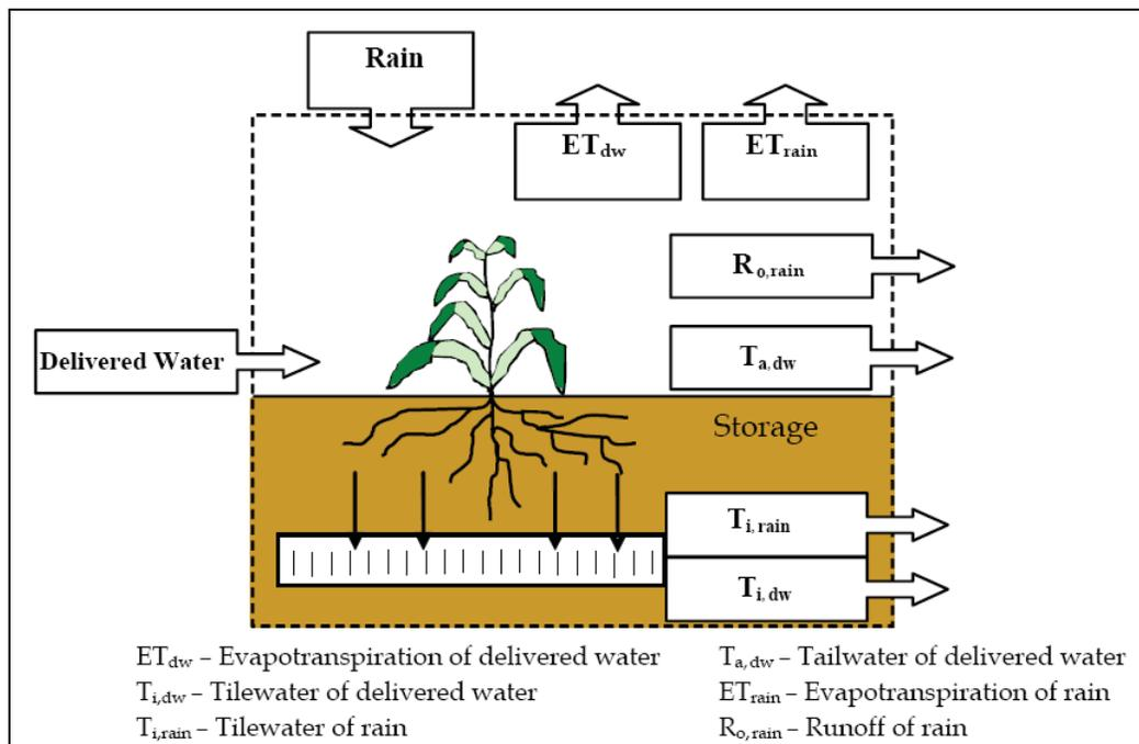
Figure 1. Conceptual Diagram of On-Farm Flow Paths.
